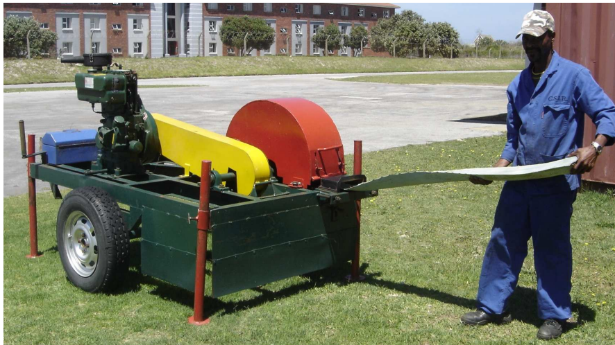
Figure 2.1. Modified decorticator for extraction of Agave fibre
